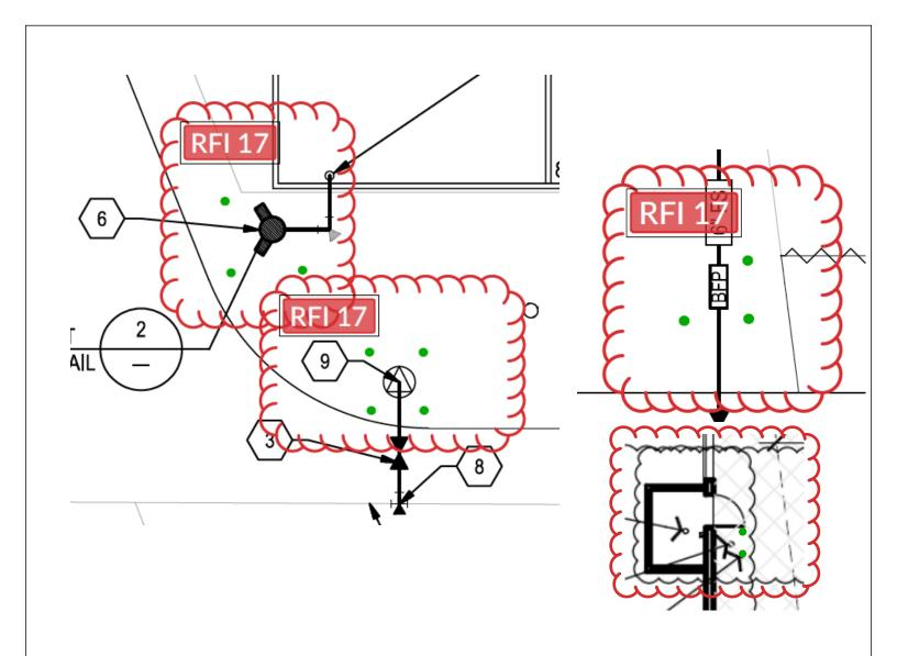
BOLLARDS SHALL BE PLACED AT THE TRAFFIC SIDE OF EACH OF THE ABOVE GROUND FIRE PROTECTION COMPONENTS (AS SHOWN ABOVE, IN GREEN) EXCEPT THAT THE HYDRANT SHALL HAVE A TOTAL OF 4 BOLLARDS PLACED AT CORNERS. HYDRANTS SHALL BE PLACE A MINIMUM OF 3'-0" FROM THE COMPONENTS WITH NOT GREATER THAN 6'-0" SPACE BETWEEN ANY TWO ADJACENT BOLLARDS.
