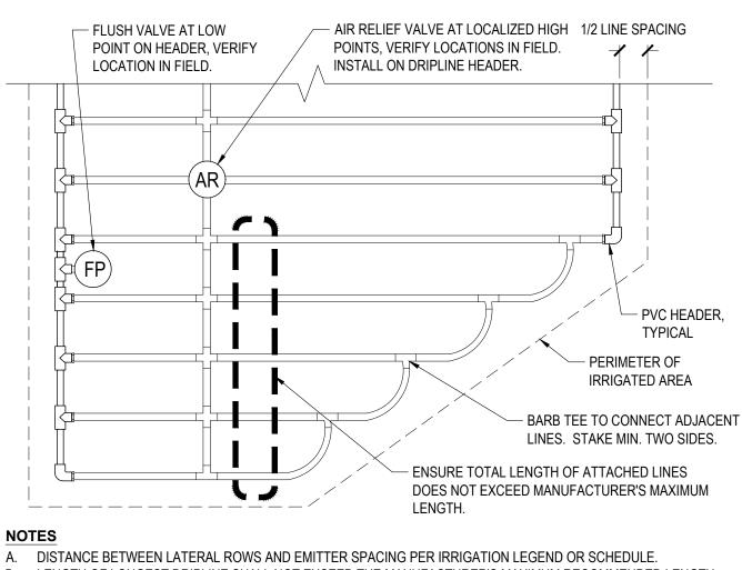
LENGTH OF LONGEST DRIPLINE SHALL NOT EXCEED THE MANUFACTURER'S MAXIMUM RECOMMENDED LENGTH. AIR RELIEF VALVE TO BE INSTALLED AT EACH LOCALIZED HIGH POINT. VERIFY LOCATIONS IN FIELD AND INSTALL
