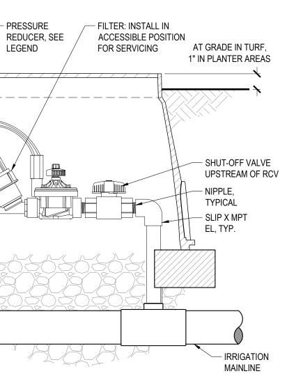
B. ALL THREADED CONNECTIONS SHALL RECEIVE 3 WRAPS TEFLON TAPE. ALL THREADED RISERS AND NIPPLES
