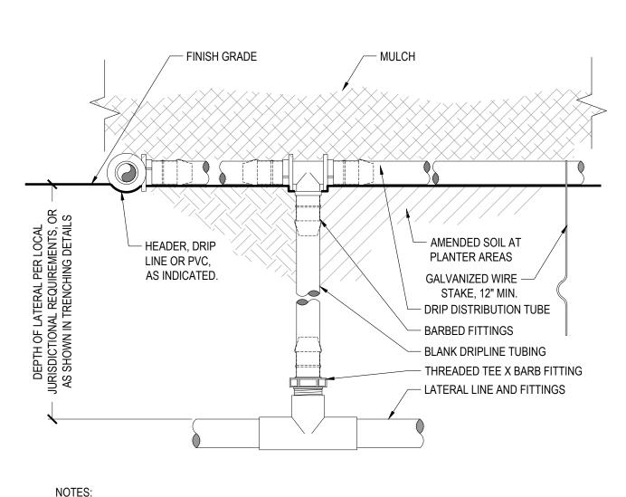
PLACE STAKES EVERY THREE FEET IN SAND, FOUR FEET IN LOAM, AND FIVE FEET IN CLAY. AT FITTINGS WHERE THERE IS A CHANGE OF DIRECTION SUCH AS TEES OR ELBOWS, USE STAKES ON EACH LEG OF THE CHANGE OF DIRECTION.
