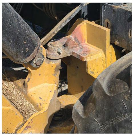
Metal fatigue between boom arm and tractor (orange/red discoloration with additional welds)
