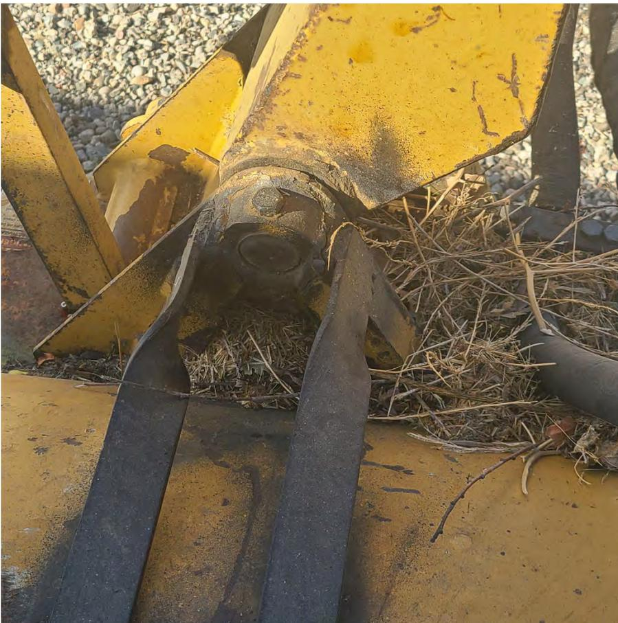
**Metal fatigue – flail mower. Additional “straps” (non-yellow bars) have been welded over the top of the flail mower to give the mower additional rigidity**
